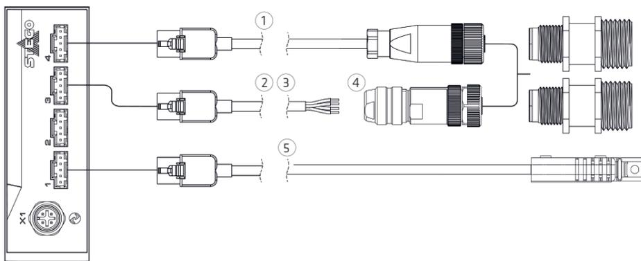
The illustration shows the IO-Link Sensor Hub SHC 071 with different sensors and connection cables (from top down):
